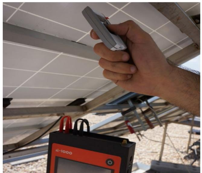
Figure 5.5. Temperature measurement via E-Temp.
