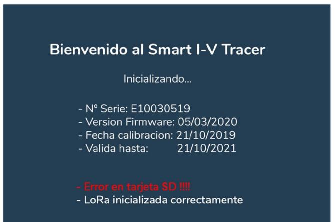
Figure 5.2. Startup Screen with SD Card Error.
