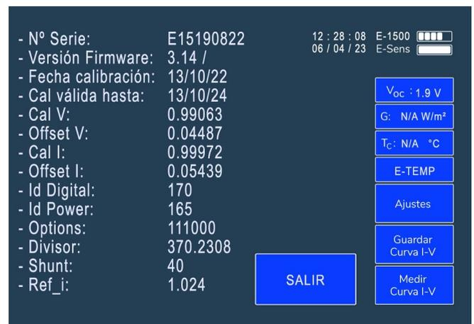
Figure 5.24. Info Button. Displays information about software and hardware.
