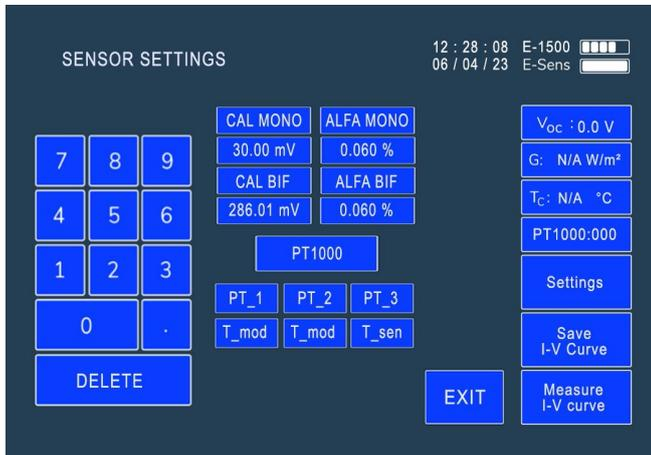
Figure 5.18. "Sensor Settings" submenu, configured for IR Sens.
