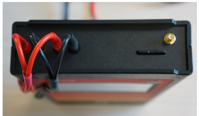
Figure 4.3.b. Incorrect connection to E-1000.
