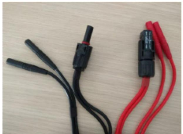
**Figure 6:** An example of a (positive and negative) cable set for the four-point probe measurement. At one end, both cables connect to the MC-4 connector and at the other end each cable connects to an isolated male banana connector.
