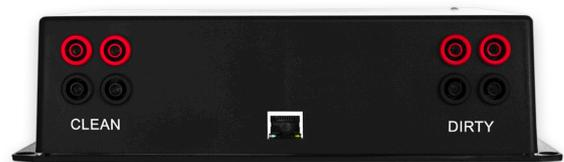
**Figure 3:** Front peripherals, including: four banana socket connectors for the clean module, four others for the dirty module, and an RJ-45 connector for an Ethernet connection. The red connectors are for the positive pole and the black connectors for the negative pole.
